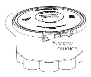
**STEP 5: FINAL INSPECTION**Screw on the knob and tighten.
