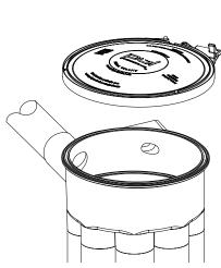
**STEP 1: TURN OFF PUMP**Before unscrewing the band clamp from the valve turn off the pump and allow for the system to depressurize.
