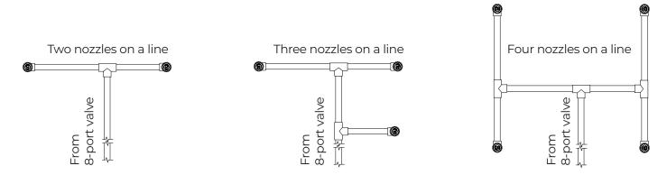
Install 2" sch. 40 PVC, 15" riser and 2"-90° elbow at each nozzle location. Risers must maintain a 90° angle to the finished pool floor. Glue 2" cap on the open end of each riser to seal for pressure test. In areas where the floor is not level, combine a 90° sweep elbow, a 45° standard elbow, and a length of pipe between the two fittings to maintain a 90°
