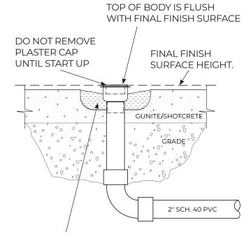
FILL WITH CONCRETE TO ½" BELOW WATER STOP FLANGE PRIOR TO INSTALLING POOL FINISH OR FILL WITH POOL FINISH
